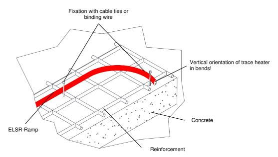
The maximum allowed heating circuit length must not be exceeded! Instead, add another heating circuit if required! Install the end termination kit as soon as possible; Under all circumstances avoid ingress of water or moisture in the trace heater. Fix end termination to reinforcement via cable ties. Trim cable ties along the entire trace heater.
